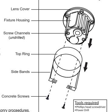
**4-** Please, support the fixture in the desired position using standard masonry proceedures.
